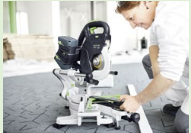
Transfer the angle accurately. Thanks to the precise angle setting on the KAPEX, the desired cutting angle can be transferred accurately with the bevel.
