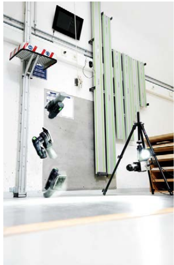
↑ During testing in Wendlingen, Festool cordless manual sanders must withstand relentless drop testing.
