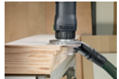
Chamfering plastic or solid wood veneer.
