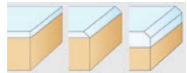
Flush Chamfered Flush + chamfered
