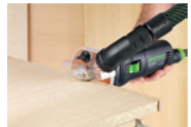
Flush trimming of plastic or solid wood veneer.
