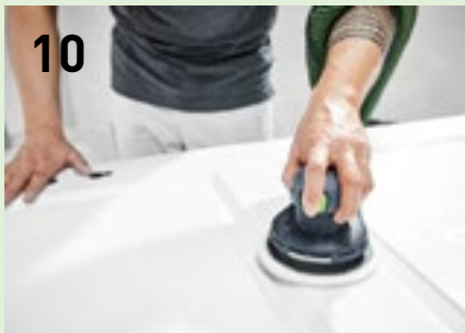
Carry out intermediate sanding using the ETS EC and an abrasive with grit (P240-P500); reduce the speed to avoid sanding through or heating up the primed surface.
